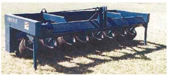
Chopper uses spinning rubber tires to pull stalks out by the roots and then chops them up with a drum-type chopper that follows behind.
