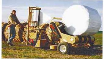
Self-loading, self-propelled bale wrapper is powered by a front-mounted 5 hp Briggs & Stratton gas engine direct-coupled to a two-stage hydraulic pump.
