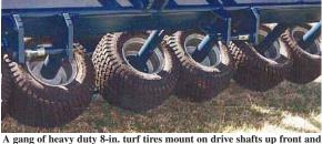
are chain-driven off a ground-driven gearbox on the machine's left side.
