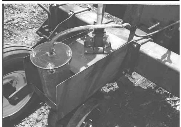
A 6-in. dia. "air canister" mounts directly above gauge wheels and has an air bag inside that's filled by a pump. Air bag applies constant downpressure to entire row unit.
