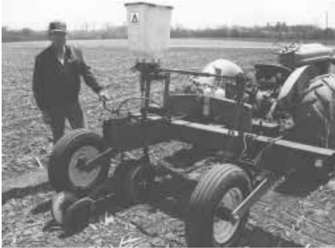
Litchfield tested his "air pressure" planter last spring, mounting a 1-row experimental unit on a short length of planter toolbar. Air pressure is used to force disc openers into the ground as well as to apply pressure to closing wheels.
