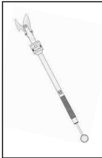
Unit has dual hydraulic cylinders. A small piston in the handle is coupled to a large piston on the cutting shears, producing a 20:1 mechanical advantage for pruning limbs up to 1 1/2 in. thick. Also available in shorter, lopping shears.
