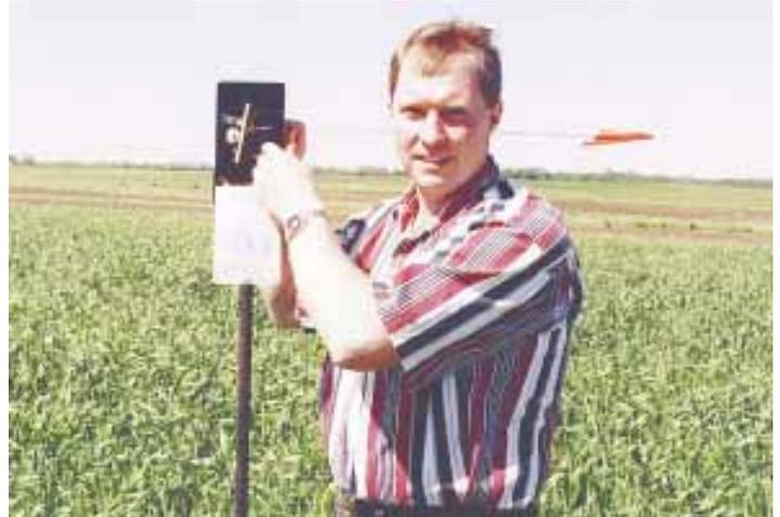
A mousetrap connects to the vacuum gauge of a conventional tensiometer. When the trap is triggered by the gauge, it raises a surveyor's flag, which can be seen from afar.
