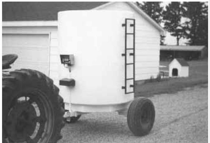
The 1,000-gal. fuel tank is fitted with an electronic scale off a grinder-mixer.
