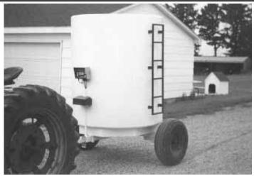
The 1,000-gal. fuel tank is fitted with an electronic scale off a grinder-mixer.
