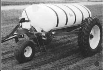
Big tires provide flotation and roadability, while the sprayer's low profile allows you to see the equipment you're pulling.
