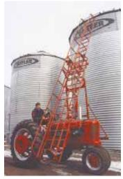
Ladder consists of two 13-ft. sections, with the inside one mounted on rollers so it can move up and down. Maximum height is 24 ft.
