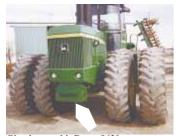
Gieseke uses his Deere 8630 tractor to apply anhydrous ammonia. He mounted a toolbox on front of it where he keeps extra anhydrous knives.
