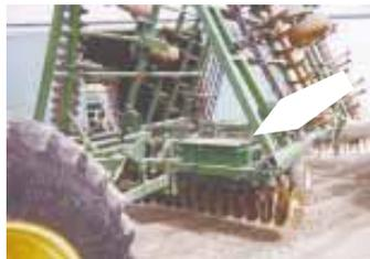
Disc-mounted toolboxes (above and left) carry sledge hammers used to dislodge rocks that get caught between disc gangs.
