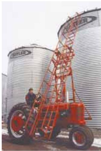
Ladder consists of two 13-ft. sections, with the inside one mounted on rollers so it can move up and down. Maximum height is 24 ft.
