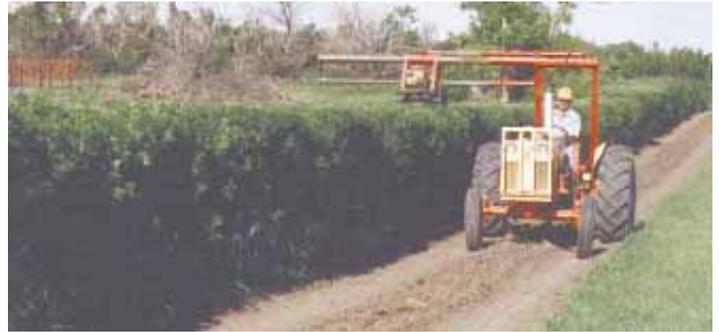
The Bonnetts made their tractor-powered hedge trimmer by mounting a 24-in. push-type lawn mower on back of their Case tractor.
