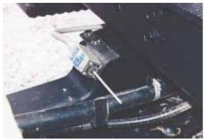
Cutoff switch automatically shuts off power to front axle whenever you turn at end of field. Kit includes front axle-mounted microswitch and "activator brackets" that mount on steering drag link.
