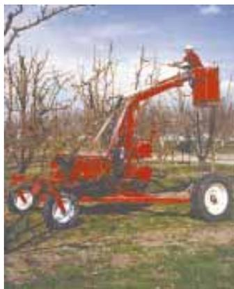
When pruning trees, McMullen drives the machine between two rows of trees and is able to trim both sides easily with his 72-in. long hydraulic pruner.
