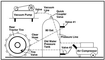
Honess pumps calcium in and out of rear tractor tires using an 80-gal. water pressure tank, a milk line vacuum pump, and a standard air compressor.
