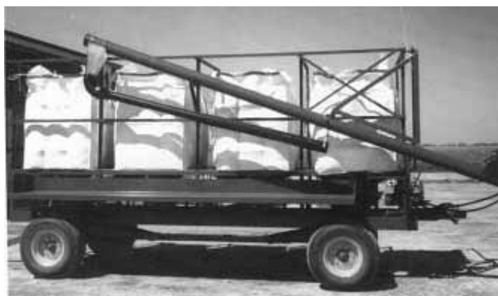
Four hoppers empty into a horizontal auger that carries seed to an 18-ft. drill-fill.
