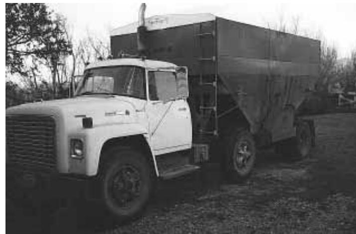
Handke mounted a 550-bu. Killbros gravity wagon on back of an International 1850 truck equipped with 466-cu. in. diesel engine.
