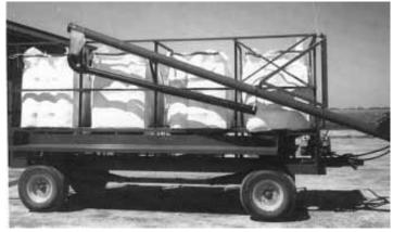
Four hoppers empty into a horizontal auger that carries seed to an 18-ft. drill-fill.
