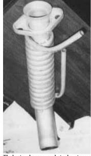
The heat exchanger uses hot exhaust gases to heat engine coolant for faster warm-ups in cold weather.
