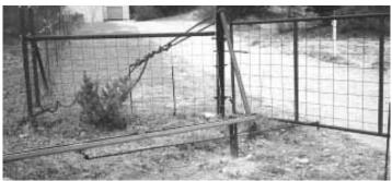
Opener pushes and pulls on a 10-ft. rod to open and close gate.
