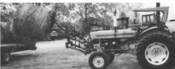
Front bale mover uses an extension designed for a rear-mount 3-pt. A heavy-duty frame that supports the bale spear.
