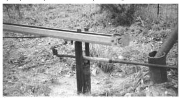
Opener mounts about 2 ft. off the ground on a pair of steel pipes.
