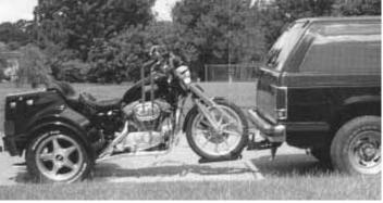
Cycle hauler completely eliminates the need for a trailer. It fits over existing trailer hitch.
