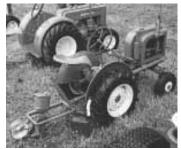
Prom's L with 1-row planter is powered by a 5 hp Briggs & Stratton engine with 3speed transmission
