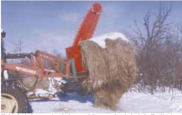
To load a bale you raise the bar straight up and stab the bale. To slice it up, you simply start the cutter chain and lower the bar onto the bale.
