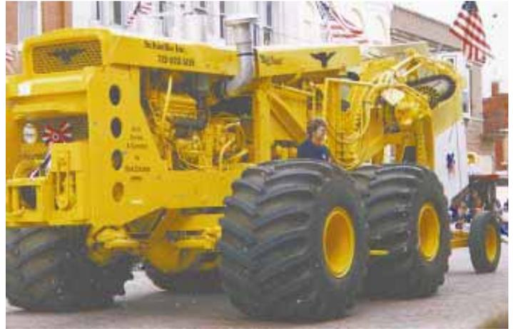
The 13-ft. high self-propelled tiling machine rides on 43-in. wide, 66-in. high flotation tires and weighs 50,000 lbs. It can dig 7 ft. deep.
