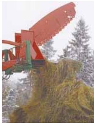
Bale can be sliced up in the air so that the loose hay falls right into a feeder.
