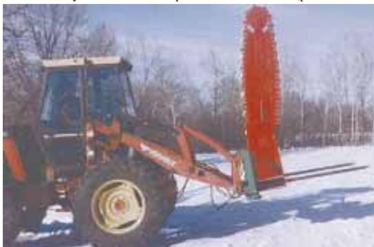
Bale cutter consists of a pivoting 6-ft. long bar and chain operated by a hydraulic motor, mounted above two bale spears.
