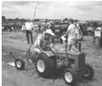
The D is powered by an 8 hp Kohler gas engine. Prom built a 4-bottom moldboard plow for the tractor.
