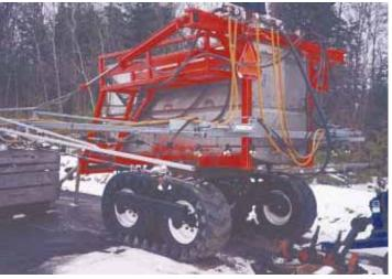
The 75-ft. wide sprayer rides on 15-in. wide, 50-in. long Goodyear rubber tracks that wrap around two 20.8 by 38 tires on each side.
