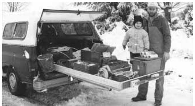
**Brian R. Hebden, Springville, N.Y.:** "I have easy access to my tools thanks to this pull-out tool tray which I built into the back of my pickup. The tray slides in and out of the bed. I used 2 by 4's and a sheet of 4 by 8-ft. plywood to make the tray. Garage door hangers and caster wheels underneath the tray
