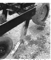
Ripper is equipped with 7 44-in. long shanks fitted with 3-in. teeth.
