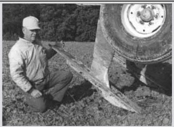
Ross Lay of Litchfield, Ill., built deep ripper he calls a "spader". It's fitted with 4-ft. blades off a road grader mounted at an angle and running 5 ft. apart. Lay runs his ripper 26 to 32 in. deep, pulling it behind a 350 hp tractor. The ripper pulls up 8-in. ribbons of claypan subsoil. Yield checks have shown a 30 bu. advantage in corn and a 6 bu, advantage in sovbeans.
