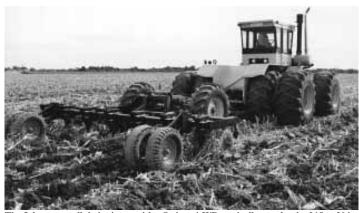
The Johnstons pull their ripper with a Steiger 4-WD, typically at a depth of 18 to 20 in.
