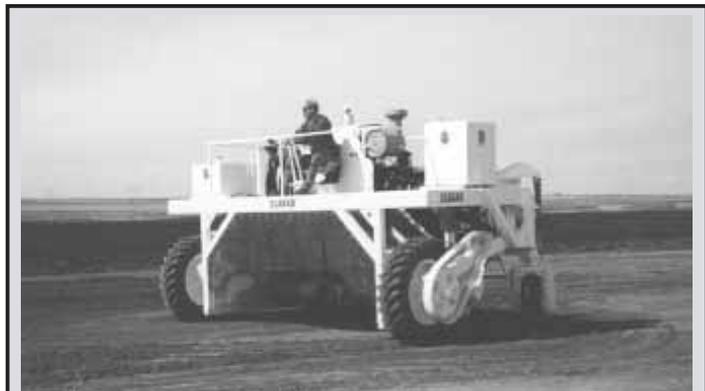
Scarab's new self-propelled turner is designed for smaller operations. It's competitive with pull-type machines because tractor isn't needed, the company says.
