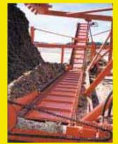
Shaft that rolls up plastic is positioned above conveyor so all remaining silage drops onto conveyor as plastic is rolled up.
