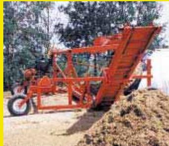
Conveyor drops silage into waiting feed truck or wagon, greatly reducing the amount of labor required to unload silage bags.
