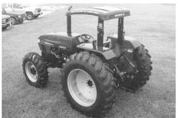
Canopy is made from a ceramic material that reflects heat better than fiberglass.
