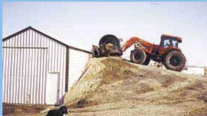
Bales are loaded into burner with a grapple fork on Klimack's tractor and are ignited with a torch from ash pit below.
