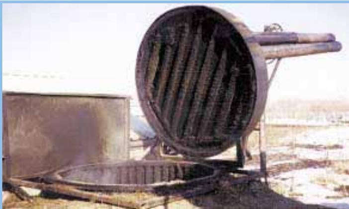
Bale furnace's 6-ft. dia. firebox is designed like a giant cage, with 48 vertical pipes spaced 2 in. apart around the outside. Lid has two 8-in. dia. smoke stacks on top.
