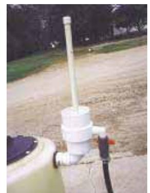
A 17-in. long piece of 1-in. dia. PVC pipe extends upward and has holes drilled in it at regular intervals. Empty containers slip over the top of pipe, which is fitted to an elbow that extends out to the side. The elbow hooks up to a water hose. The rinse water."
