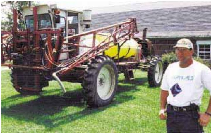
Charles Corzatt and his hired man, Greg Deitrich, used components from two IHC 715 combines and a New Holland TR 70 combine to build the sprayer. It has a 60-ft. boom.
