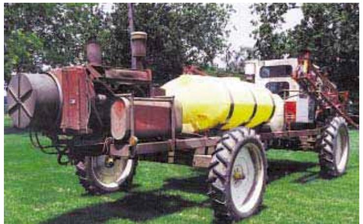
They used the front axle and cab off one of the 715's and the motor and hydrostatic drive off the other. Rear axle is off the New Holland combine. Note 750-gal. spray tank.
