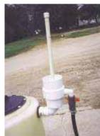
A 17-in. long piece of 1-in. dia. PVC pipe extends upward and has holes drilled in it at regular intervals. Empty containers slip over the top of pipe, which is fitted to an elbow that extends out to the side. The elbow hooks up to a water hose. rinse water."
