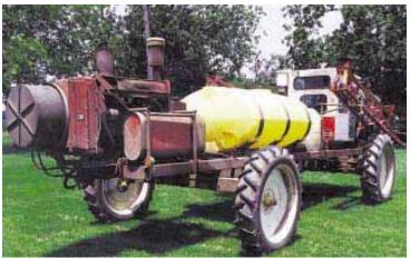
They used the front axle and cab off one of the 715's and the motor and hydrostatic drive off the other. Rear axle is off the New Holland combine. Note 750-gal. spray tank.
