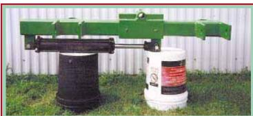
"Slider hitch" hydraulically shunts pull-type planters over to the right or left, up to 8 in. That way you can avoid having to drive over last year's rows.
