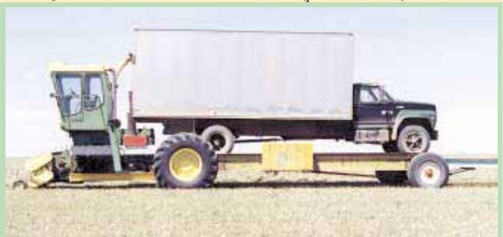
Forage harvester's spout actually extends inside the truck. Note big flotation tires on front of trailer and hydraulic-operated dovetail ramp on back.
