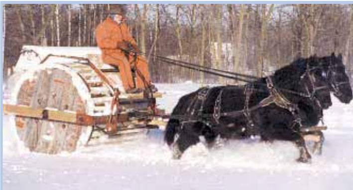
Homemade "snow packer" creates a 6-ft. wide trail for sleighs. It was made out of a 6-ft. wide, discarded wire reel from a utility company.
