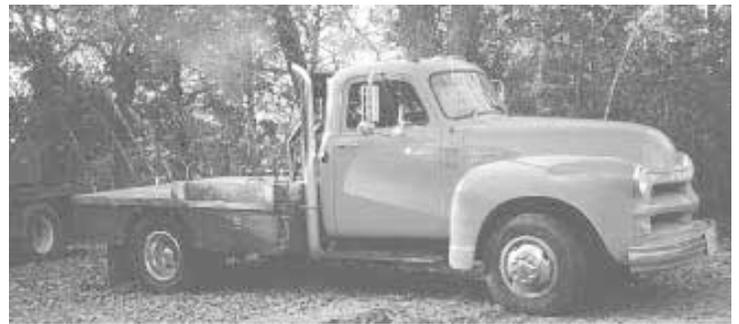
Draehn installed a 256 cu. in., 4-cyl. turbocharged diesel engine - out of a 1976 Ford 77 tractor - in this 1954 Chevy S4 1 1/2-ton pickup. "It really has pulling power," he says.
