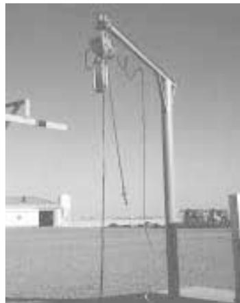
Home-built slaughter system starts with this 15-ft. high electric-powered hoist equipped with a 10-ft. long arm on top that's free to rotate 360 degrees. Hoist rolls back and forth on arm.
