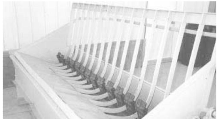
Electric-powered hair remover consists of a 10-ft. long steel tub with a powered shaft at bottom that's fitted with rubber flaps. Animal is lowered to bottom of tub by a steel cradle with rods spaced 3 in. apart. The rubber flaps come up through the bars on the cradle to remove the hair.
