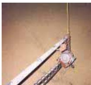
End of track inside bin is supported by a rope connected to top of bin.
