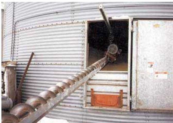
Nuehring attached 18-ft. long section of roller track off a sliding door to top of bin's door frame. He uses the track to roll auger inside the bin.
