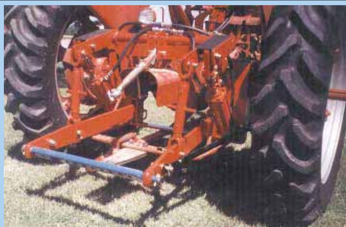
On International Harvester tractors the add-on 3-pt. hitch is raised and lowered by
