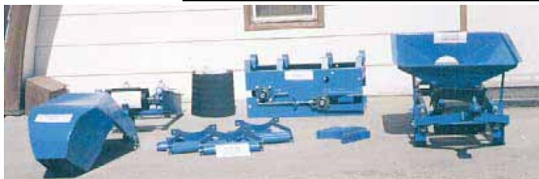
Conversion kit consists of both top and bottom roller drive units. The top end is equipped with a discharge spout and the bottom end is fitted with a 36-in. sq. hopper. There are also belt return rollers and brackets that mount underneath auger tube every 4 ft.
