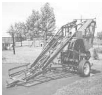
Unit is also available as a hydraulically-operated model on wheels that automatically lays down a Zimmie stack.
