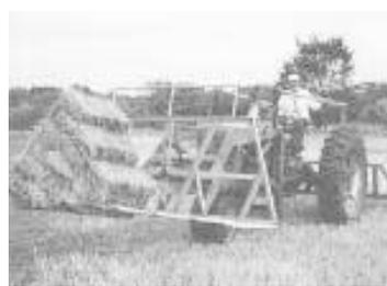
Bales can be easily transported with this loader-mounted stack handler.
