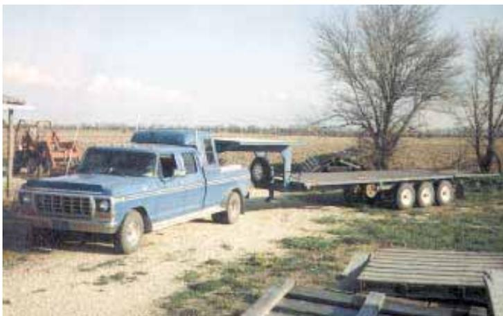
Regier repowered his 1978 Ford F-350 1-ton pickup with a 429 cu. in., V-8, 368 hp gas engine. He uses it to pull a 36-ft. long gooseneck trailer that has an extra 8-ft. deck over the gooseneck and an 8-ft. hydraulic-operated dovetail ramp on back.
