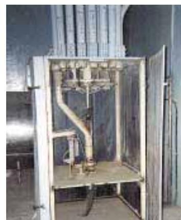
At the home-built feed distributor the pipes come together in a circle. Computer automatically rotates movable "arm" on distributor to connect it to the proper pipe. Close-up of distributor (below) shows electrical contacts that control the system.
