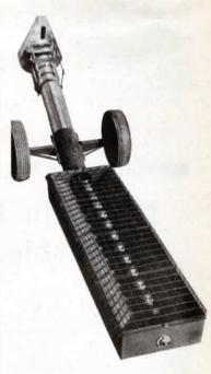
Low profile hopper (11 in. high) fits under "Bobtails" and bottom-dump trucks. Unloads 2,250 bu. of dry grain at 549 rpm. Powered by 5 hp electric motor.
