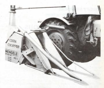
Capacity of Model MB3 is up to 40 tons per hour. Mounting crossbar is equipped with a hitch support and towing hitch. Machine quickly and effortlessly attaches to tractor's 3-pt. hitch.
