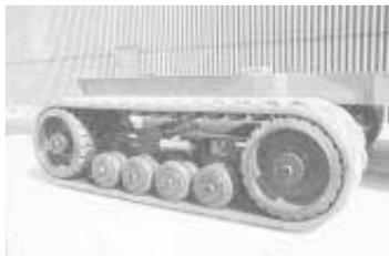
**The 70-in. long system exerts just 7 psi of ground pressure with a 20-ton load, company says.**
