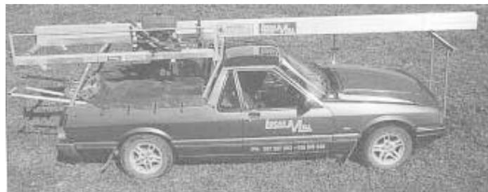
**Portable saw mill can be transported on a utility vehicle or pickup.**
