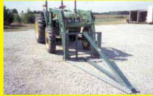
FARM SHOW readers might be interested in this loader-mounted saw that I built to cut trees. It's ideal for quickly ripping through trees 3 in. in dia. and less but works on much larger trees. too.
