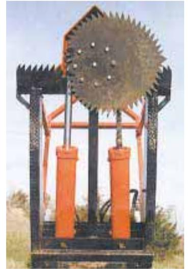
Toothed saw blade is attached to a pair of hydraulic cylinders that rotate blade into tree. Half the teeth on blade point in one direction and the other half point in the opposite direction.
