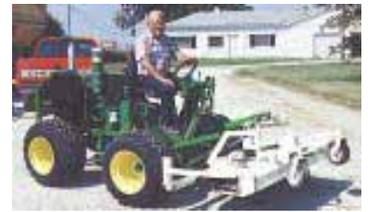
Home-built mower is powered by a Sundstrand hydrostatic motor for easy maneuverability around trees, buildings.
