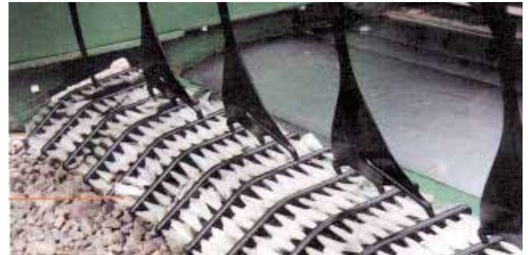
"Bean Sweep" consists of two parts - lifter bristles mounted on the sickle guards and optional poly paddles that mount on pickup reel.
