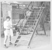
from side to side so that all four wheels carry an equal load on uneven ground. To reduce any danger of tipping, threaded adjustment cranks can be used to tighten down either end of the axle and make it rigid.
