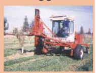
Tree-trimming attachment was built by mounting a swather sicklebar on an old forklift mast. It reaches up to 12 ft. high.
