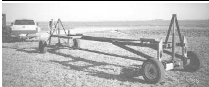
**Hydraulic cylinders operate with a hand pump located on front of the cart.**
