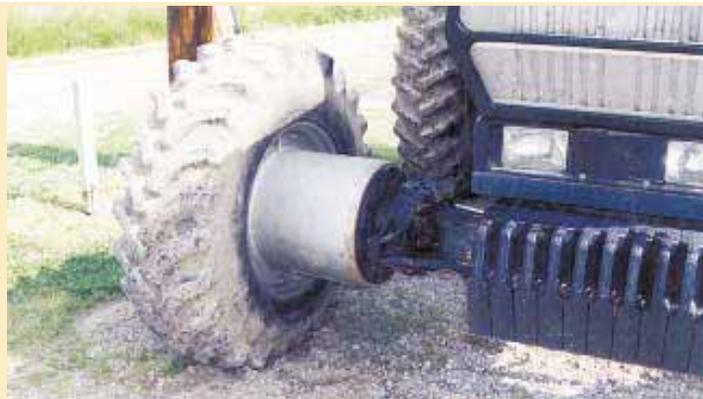
Welder Gary Hatten made "spacers" from 16-in. dia. oil field pipe. "Spacers" move front wheels out so they run in line with the outer duals on back of tractor.
