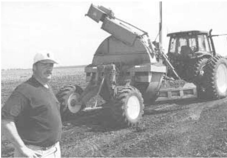
Watershed Management's ditcher has been totally reengineered into a pull-type unit.
