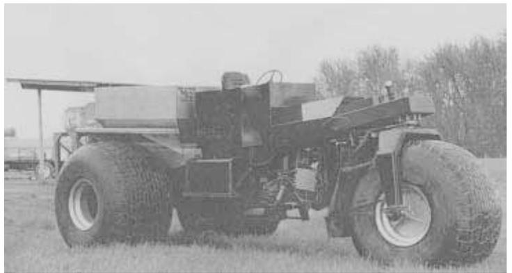
Riding on 66 by 44-in. flotation tires, the rig can be used either as a fertilizer spinner spreader or as a sprayer.
