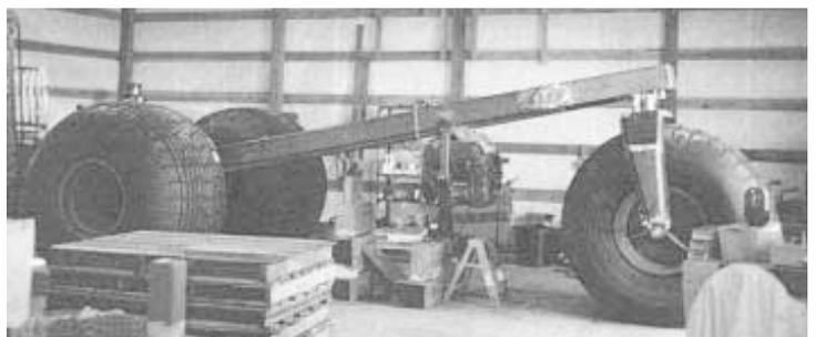
A single length of 2 by 8-in. steel tubing was used to build the frame.
