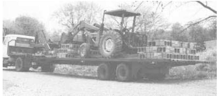
With rack removed the flatbed trailer can be used to haul conventional loads.
