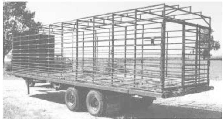
Rack will hold 18 to 20 head. When not in use for hauling cattle, rack is simply stored on the ground out of the way.
