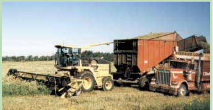
Custom forage harvester Dan Prefontaine mounted a 25-ft. Honey Bee header on his New Holland FX45 self-propelled forage harvester. Silage is blown into a 15-ton Jiffy "accumulator box" which unloads on-the-go into tandem axle trucks.
