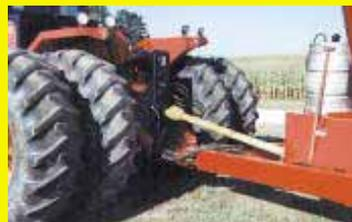
Beer keg bolted to auger wagon serves as a 15-gal. gas tank for the add-on engine.
