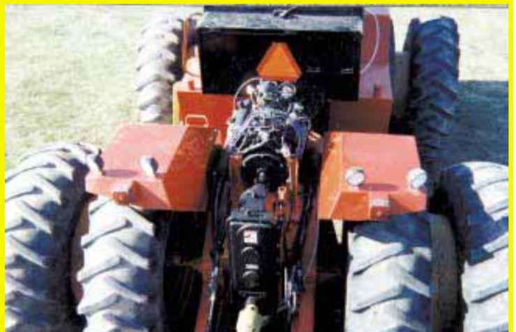
Engine shaft-drives a drop box with a self-contained clutch pack off a 1970's Case 4-WD tractor. A hydraulic cylinder engages the clutch pack to turn the pto on or off.
