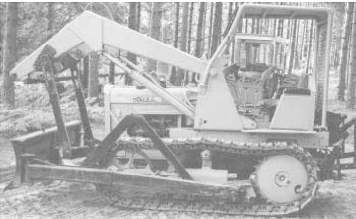
Fifelski's International crawler loader is fitted with the blade off a 1010 Deere dozer.
