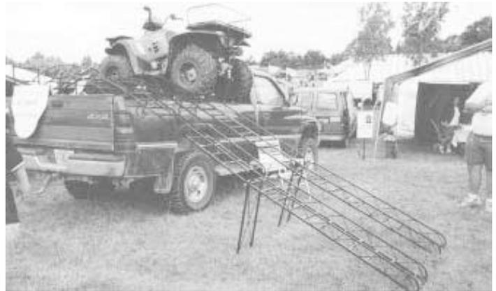
Ramp system consists of four separate steel arches that mount in pickup bed. Side ramps run from ground up to pickup.
