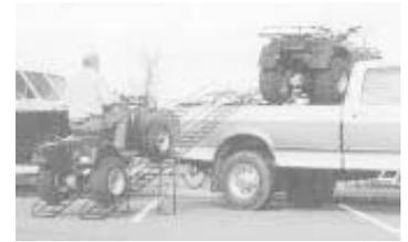
You drive ATV onto one set of arches and secure it, then move the ramp over and drive the second ATV up.
