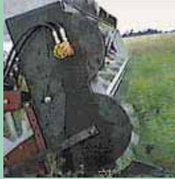
"Clean Cut" attachment consists of two 18-in. rotary blades fitted with sickle sections.
