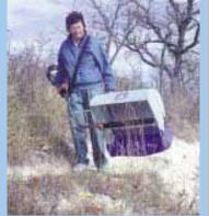
Hand-held seed harvester mounts on a Stihl string trimmer powered by a 2-cycle gas engine. Head was removed and replaced by an 18-in. long nylon stripper brush that strips seeds off.
