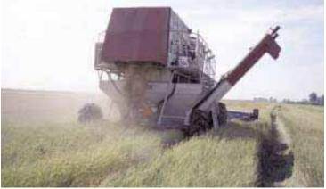
Unlike other combines, grain tanks are located at the bottom of the units which lowers the center of gravity and eliminates the need for elevators.
