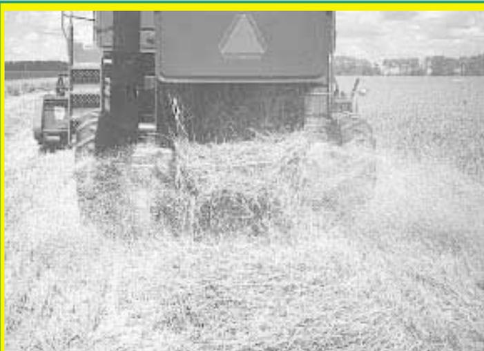
Home-built chaff spreader allows Glanville to put straw in a windrow for baling. He can spread chaff at the same time.
