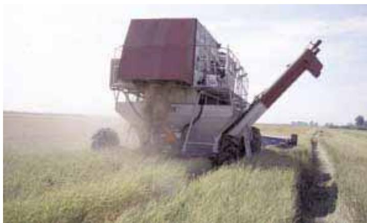
Unlike other combines, grain tanks are located at the bottom of the units which lowers the center of gravity and eliminates the need for elevators.
