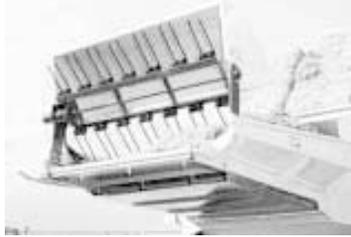
Long steel tines rotate around a hydraulically-powered shaft.
