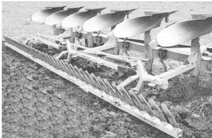
The moldboard plow-mounted "Furrow Cracker" mounts on the side of the plow to break up clods and level seedbeds at the same time.
