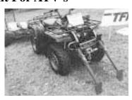
Kit includes an anchor, base plate, two stool legs, and an electric drum winch that mounts on the base plate. It's remote-controlled so the operator can stand clear of the cable and ATV during winching.
