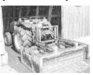
Scraper is equipped with two steel blades with pivoting rubber squeegee ends.
